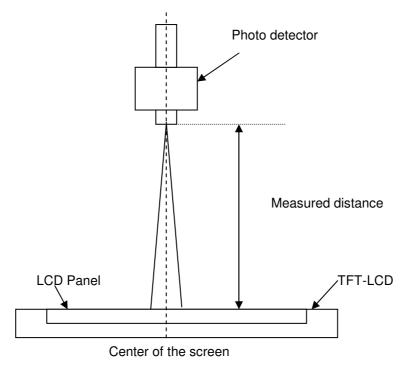
**Note 2:** Definition of viewing angle measured by ELDIM (EZContrast 88)
